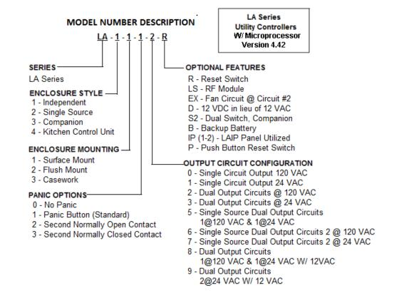
NOTE: Output Configurations 5, 6, 7, 8 and 9 are intended to operate with specific operators and solenoids for applications such as Instructor's Demonstration Stations and Science Preparation Rooms. When Configurations 2 or 3 are specified with Single Source Units, then Outputs are typically provided as single switch operators with or without a Reset per each output.
